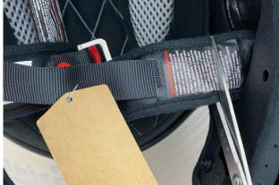
**Step 5)** Place the two cut straps (one of them will include E13 ECE serial number) in an envelope or a small box. Every strap needs to be packed with the corresponding RA N° (see picture below). A customer service agent will assist you with the process and will inform you when UPS will pick up the package. When received, we will issue a credit memo.
